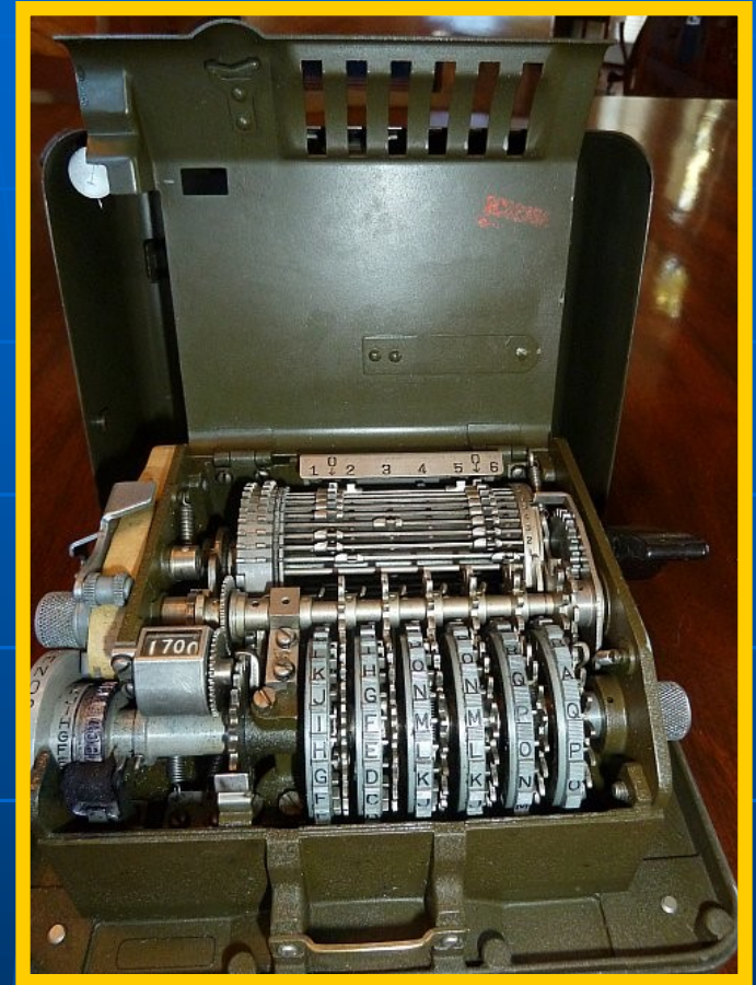
M-209 with inner lid open to reveal 6 wheels and drum
